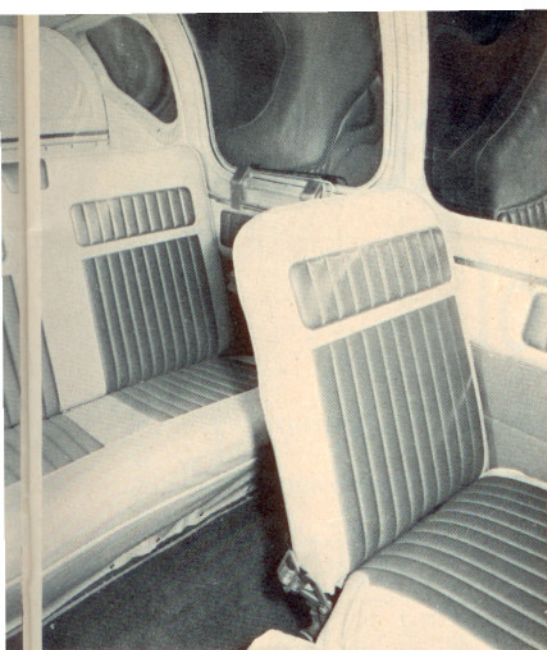
Beechcraft's El Dorado kit has simplified the installation of new interiors in Bonanzas. This is a refurbishing job that was done on an early model of the popular single-engine plane
